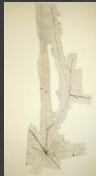
Photographic emulsion exposed to cosmic rays at high altitude
